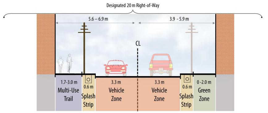
Note: Splash Strip includes Curb and Gutter
