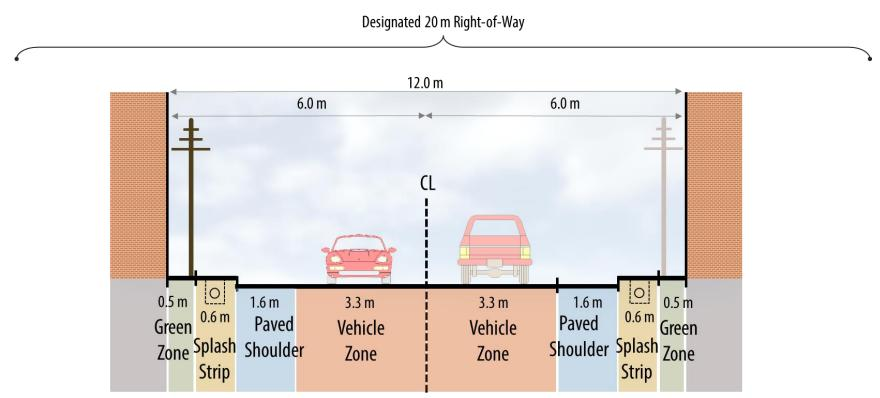
Constrained Rural Main Street (12 m Typical ROW – Sidewalk on Both Sides)
