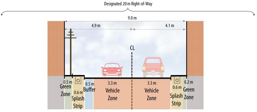
Constrained Rural Main Street (9.0 m Typical ROW – Minimal Paved Buffer on Both Sides and Minimal Green Zone)
