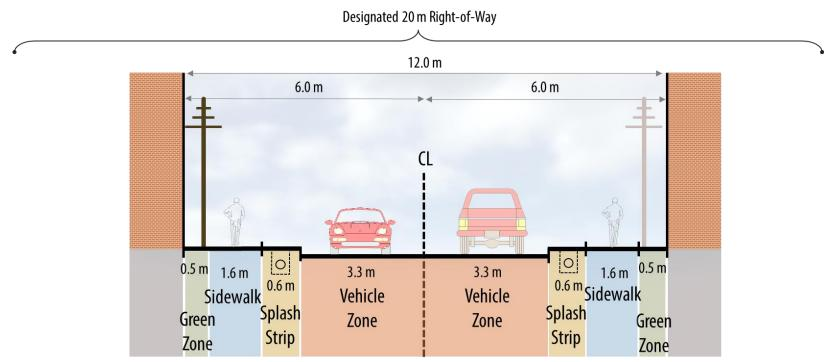
Note: Splash Strip includes Curb and Gutter
