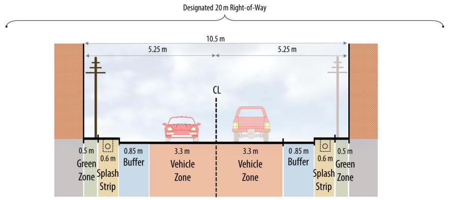
Note: Splash Strip includes Curb and Gutter
