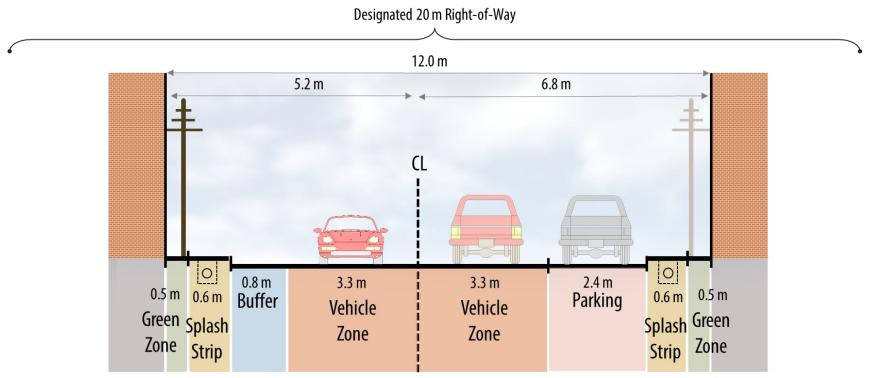
Note: Splash Strip includes Curb and Gutter
