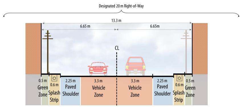
Note: Splash Strip includes Curb and Gutter
