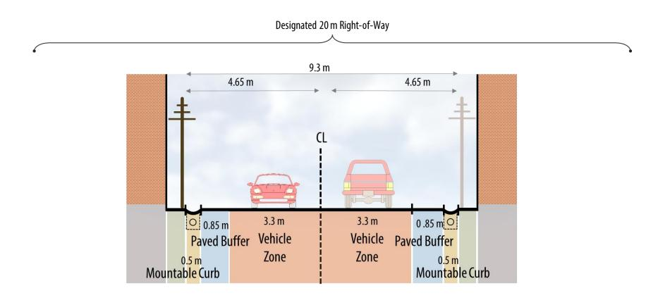
Constrained Rural Main Street (9.0 m Typical ROW – Narrow Paved Buffer on One Side and Minimal Green Zone)
