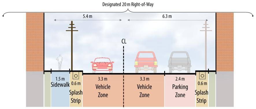
Note: Splash Strip includes Curb and Gutter
