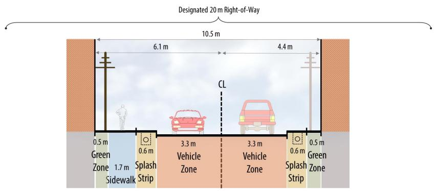
Note: Splash Strip includes Curb and Gutter
